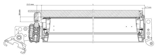
$\Delta L_{1,up,dfl}$  = -9,7 mm,  $\Delta L_{2ll,up,dfl}$  = 23,5 mm and  $\Delta L_{2}\perp_{,up,dfl}$  = 24 mm. All these measurements are constants.
